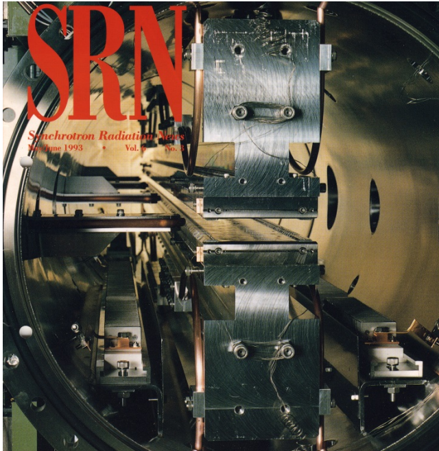
In-vac Us ( \lambda u=4\text{cm} ) @ 6.5GeV PF-AR (since 1989) Gap=10mm
