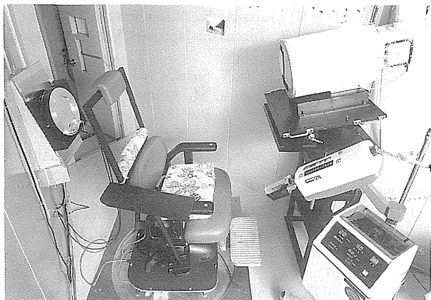
Figure 5. Inside the clinical hutch, NE1A3. An x-ray exposure-dose counter on the left-hand side, a special chair for the patient, an x-ray imaging system (II-TV), an auto-injector for contrast material can be seen.
