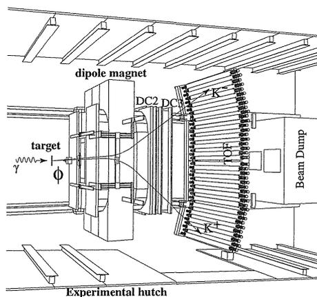
Figure 3. Top view of the spectrometer system (LEPS) in the experimental hutch. The spectrometer mainly consists of a dipole magnet, drift-chambers, and scintillation counters for TOF measurement. High-energy  $\gamma$ -rays coming from the left side are stopped at the beam dump (in the right side of the figure). A typical event of  $K^+ + K^-$  pairs for  $\phi$ -meson production is shown.
