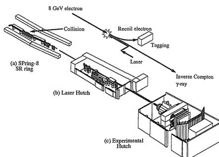
**Figure 1.** Laser-Electron-Photon (LEP) facility at SPring-8. The facility mainly consists of three parts; (a) Laser-electron collision part in the storage ring of SPring-8, (b) Laser hutch for laser injection, and (c) Experimental hutch. The recoiled electrons are tagged for energy information. A simple schematic explanation on the collision between electron and laser light is inserted in the figure.
