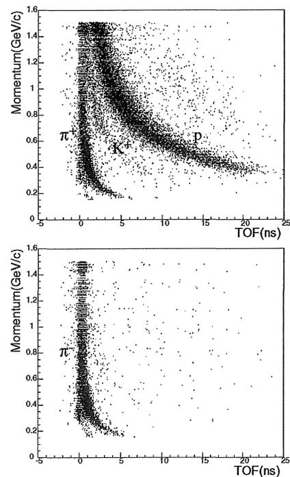
Figure 4. Scatter plot for the particle identification. (a) Particle events with positive charged particles. (b) Events with negative charges.
