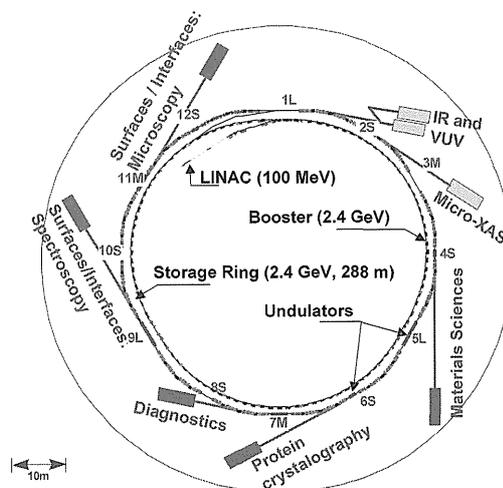
Figure 2. Schematic layout of the SLS showing linac, full size booster, storage ring, and the beamlines. Four undulator beamlines plus a diagnostic beamline are under construction, two more (shown hatched) are under design.
