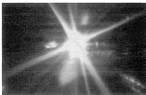
Figure 1. Image from a synchrotron radiation monitor showing the first stored beam on December 15<sup>th</sup> after only 4 days of commissioning. The beam parameters are 2.4 GeV beam energy, 3 mA current, and a lifetime of approx. 10 minutes. After 4 days, the lifetime increased to 8 hours at the same current.
