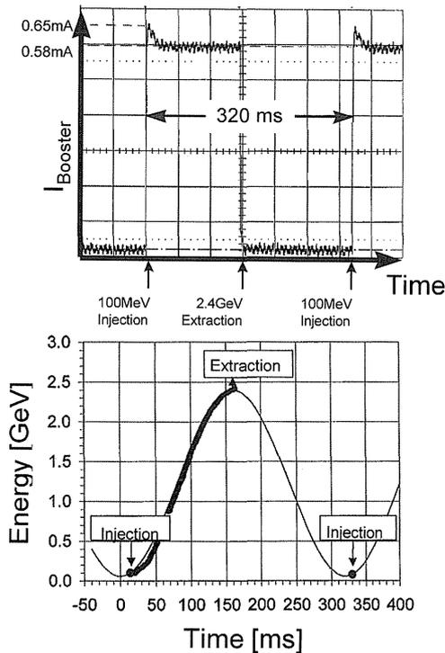
Figure 3. Acceleration cycle of the booster showing a full energy cycle (bottom) and the current in the booster during the full cycle (top).
