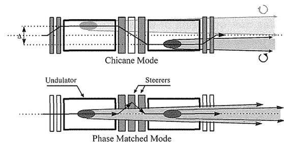
Figure 5. Schematic top view showing the helicity switching. Two undulators are located in line. The electron beam can be offset ( $\Delta \sim 1$  mm) using steerer magnets (top). This produces two separate horizontally displaced light sources. If no helicity switching is needed, the steerer magnets phase match the two undulators, thus maximizing the brightness (bottom).
