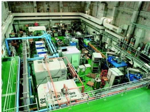
Figure 4a. Injection system of the JAERI superconducting rf linac-based free-electron laser.
