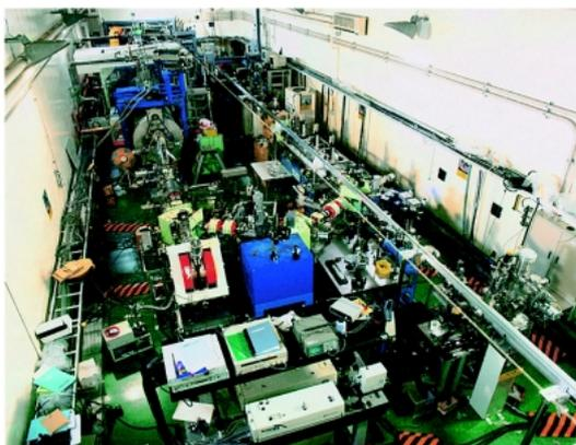
Figure 4b. Main accelerator system of the JAERI superconducting rf linac-based free-electron laser.
