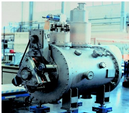
Figure 4c. JAERI compact stand-alone, and zero-boil-off cryostat module for the superconducting rf linac.
