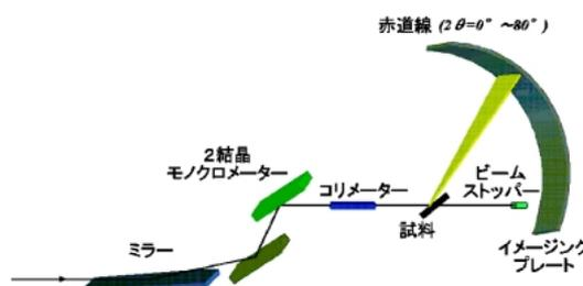
Figure 2. The schematic view of Beamline.
