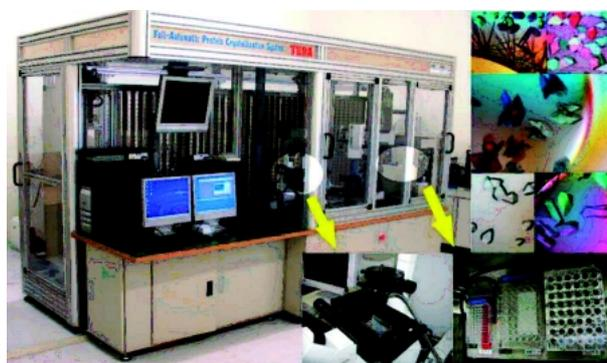
Figure 2. Full Automatic Protein Crystallization and Observation Robot System "TERA".
