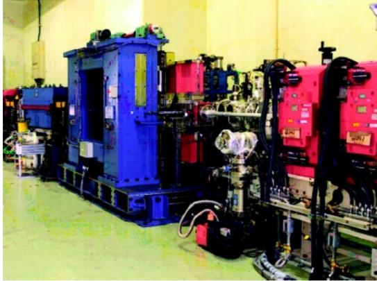
Fig. 2 Photograph around the MPW#5 after the ring reconstruction. A 1.5 m free space is created between the MPW#5 and a new pair of quadrupole magnets.
