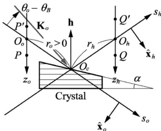
Fig. 1 Coordinate systems for incident and reflected beams.
