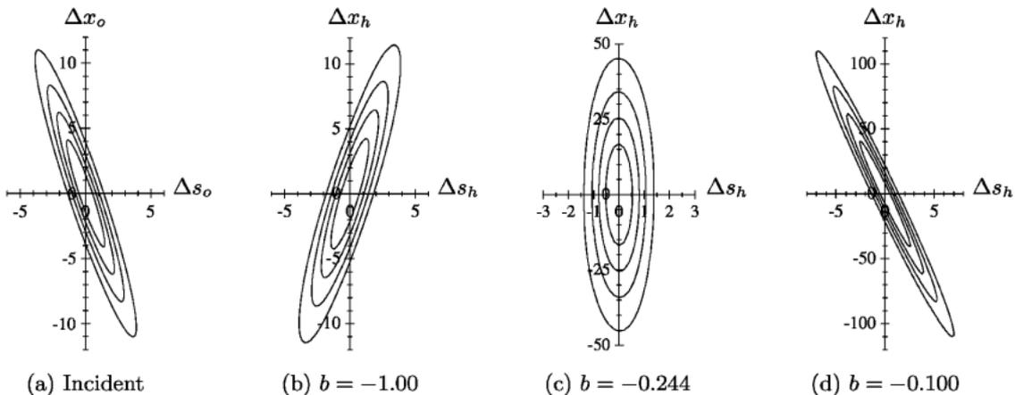
**Fig. 5** Absolute values of the complex degrees of coherence of x-ray beams reflected by silicon 111 crystals with various asymmetry factors  $b$ . (a) Spatial distribution of the complex degree of the incident beam; (b) (c) (d) ones of the reflected beams. The contours show the positions where the absolute values are 0.8, 0.6, 0.4 and 0.2, going from the inside outwards. The units of the coordinate axes are micrometer.
