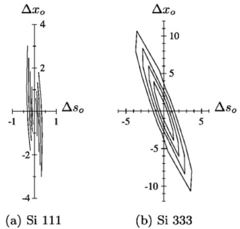
Fig. 3 The complex degrees of coherence of the x-ray beams prepared with the silicon DCM of (a) 111 and (b) 333 reflection. The contours show the positions where the absolute values of the complex degrees are 0.8, 0.6, 0.4 and 0.2, going from the inside outwards. The units of the coordinate axes are micrometer.
