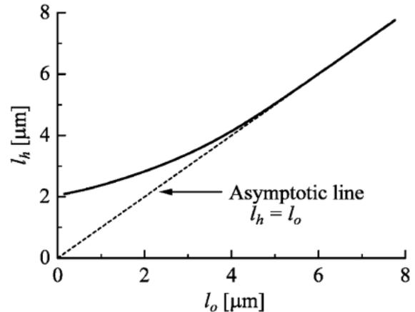
Fig. 6 Change of coherence length in the direction of the reciprocal vector. The incident beam with  $0.661 \text{ \AA}$ -wavelength,  $\sigma$ -polarization and  $l_o$ -coherence length impinges on a silicon crystal of 111 symmetric reflection to become the reflected beam with  $l_h$ -coherence length.
