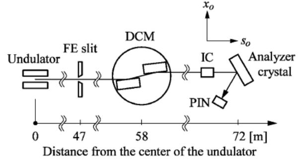
Fig. 2 Front view of the experimental setup for coherence analysis. The front-end (FE) slit was opened to the square with a side length 1 mm. An ionization chamber (IC) and a silicon PIN detector (PIN) were used for rocking-curve measurements with an analyzer silicon crystal.
