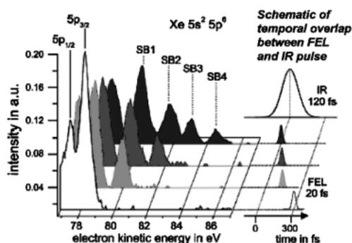
Fig. 8 Single-shot spectra in the region of the Xe 5p-1 line and the high-energy sidebands taken at the nominal temporal overlap  $\Delta t=0$  and due to jitter also at  $\Delta t \neq 0$ . The spectra are normalized to total FEL + IR intensity.
