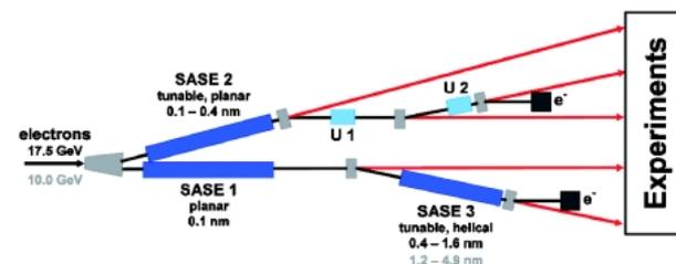
Fig. 4 Insertion devices at the European XFEL Facility and wavelength range of FEL radiation produced when operating the LINAC with 17.5 GeV or 10 GeV, respectively.
