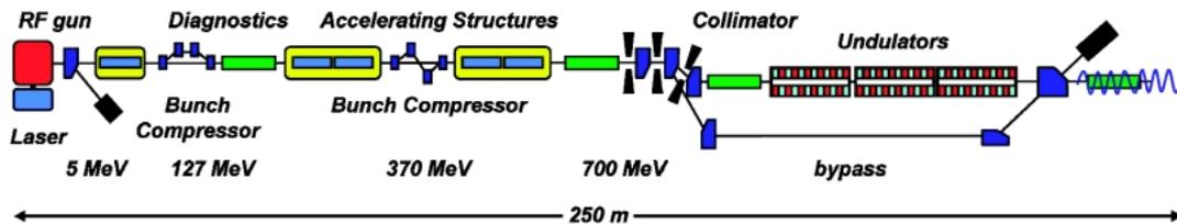
Fig. 5 Schematic layout of the accelerator part of FLASH.
