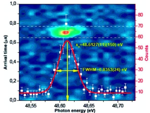
**Fig. 10** Fluorescence spectra as a function of arrival time relative to the FEL pulse and versus photon energy.
