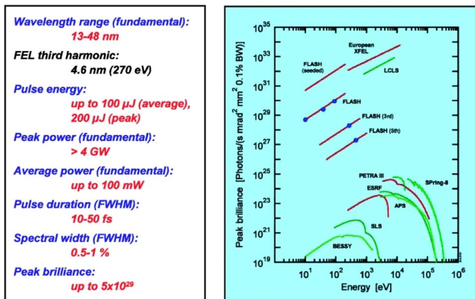
Fig. 6 Performance of the FLASH facility at DESY.
