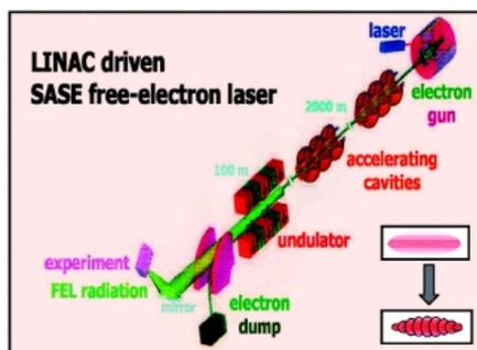
Fig. 2 Main components of a SASE free-electron laser where the originally homogeneously distributed electron charge in a bunch is transformed in a modulated structure with a period equal to the wavelength of the undulator X-rays.
