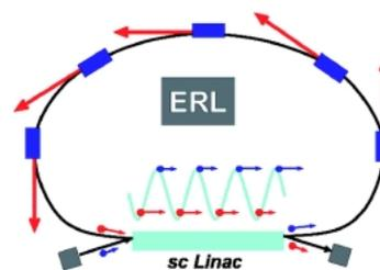
**Fig. 1** Principles of an X-ray source with an Energy Recovery Linac operated with superconducting radio frequency.
