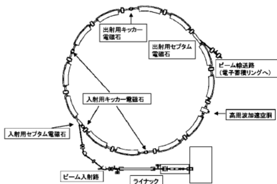
Fig. 10 Layout of booster synchrotron and linac.
