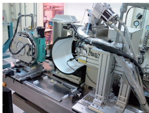
Fig. 1 A photograph of large cylindrical imaging plate (IP) camera installed at SPring-8 BL02B1.
