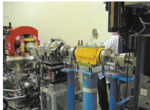
Fig. 12 Pulsed sextupole magnet (yellow-colored magnet in the photo) installed at the straight section of the PF-Ring.
