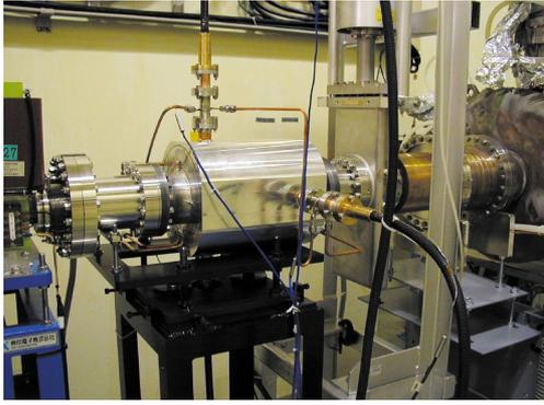
Fig. 6 Photo of longitudinal kicker cavity installed at the downstream of main accelerating cavity.
