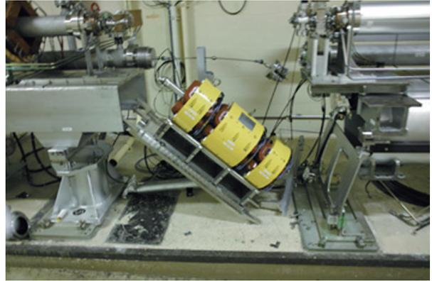
Fig. 1 (Color online) A triplet Q-magnet fell down in the linac.
