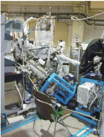
Fig. 3 (Color online) A vacuum chamber tipped over.
