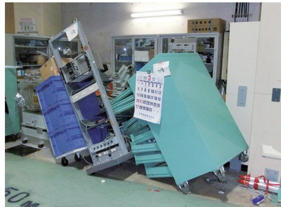
Fig. 5 (Color online) Unlocked tool cabinets dropped over and damaged neighboring equipments.
