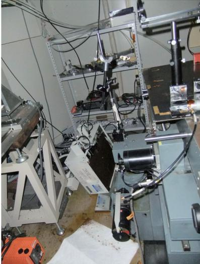
Fig. 2 (Color online) A diffractometer fell down from its support table.
