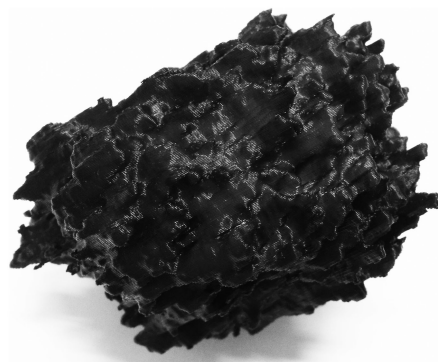
Fig. 1 Photograph of a 3D print model of a separated Mn-microparticle made from tomography images. Scanned 3D image of approximately 7 \mu\text{m} diameter Mn-microparticle is magnified by 10^4 times and printed. Sample is measured using synchrotron-based X-ray microcomputed tomography at BL47XU, SPring-8.
